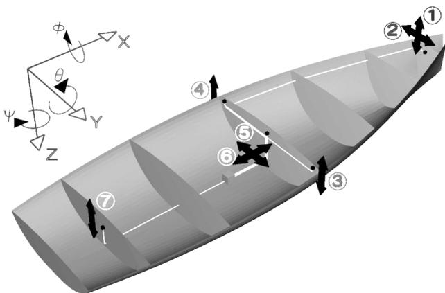
**Fig. 1** Position and sensitive axes of the accelerometers
