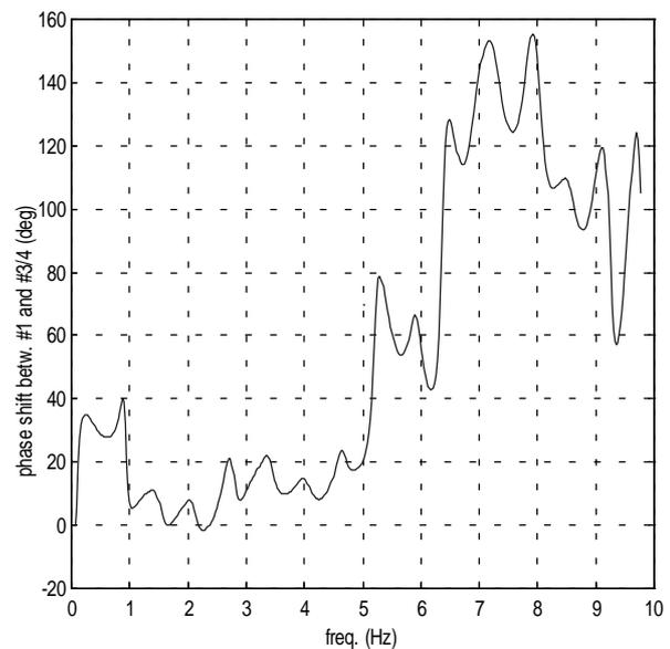
**Fig. 6b** Phase difference between the signals of accelerometers mounted at the bow and close to LCG.
